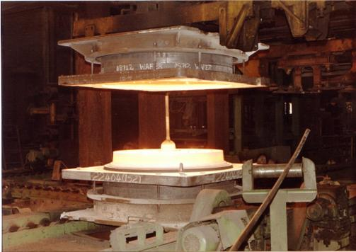
The wheel then undergoes the process of heat treatment, Cleaning, Magnaglo testing, Ultrasonic testing, Peening and various stages of inspection. The wheel produced by this process requires no machining except the precision boring of central hole (hub) where the axle has to be fitted.
